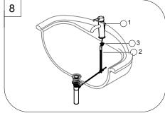
Insert lift rod (1) through faucet and into strap (2). Tighten screw (3).
