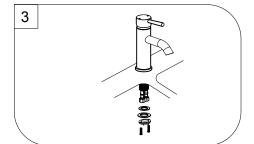
Remove the two screws from locking nut. Under the sink install the rubber washer, steel washer, and locking nut onto the shank. Tighten the locking nut with a basin wrench or socket tool and install the two screws to secure the faucet in place.
