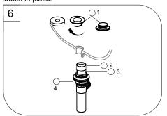
Apply plumber's putty to the underside of flange (1). Apply teflon tape to threads at the bottom of flange (1). Insert body (2) into sink. Screw flange onto body. Pivot hole (3) must face the back of the sink. Tighten nut/gasket (4), do not over tighten. Clean excess putty.
