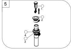
Remove stopper (1) and flange (2). Screw nut (3) all the way down. Push gasket (4) down.
