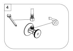
Apply pipe tape onto threads of water supplies. Use wrench when tightening the hose connection, do not over tighten.
