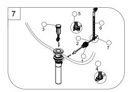
Remove pivot nut (1). Insert the stopper (3) into the drain hole and Insert horizontal rod (2) through the hole of the stopper (3) according to graphic (5). Hand tighten pivot nut (1). Attach horizontal rod to strap (6) using clip (7).
