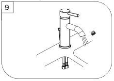
After installation is completed, turn on water supply and allow both hot and cold water to run for one minute each. While water is running, check for leaks. Reinstall aerator. Your new faucet is ready to use.
