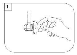
Shut off water supplies. Remove old faucet. Clean sink surface in preparation for new faucet.
