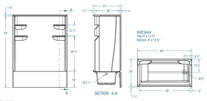
FEATURES Dimensional Tolerance ± 1/2". Dimensions needed for site preparation should be measured from the unit. Stream33 assumes no responsibility for preparatory work.
