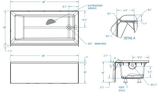
FEATURES Dimensional Tolerance ± %". Dimensions needed for site preparation should be measured from the unit. Stream 33 assumes no responsibility for preparatory work.
