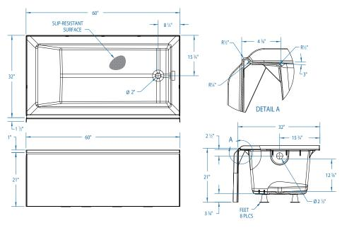
$FEATURES \qquad \text{Dimensional Tolerance} \pm \text{\%.} \text{ Dimensions needed for site preparation should be measured from the unit. Stream33 assumes no responsibility for preparatory work.}$
