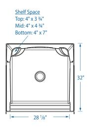
FEATURES Dimensional Tolerance ± %". Dimensions needed for site preparation should be measured from the unit. Stream33 assumes no responsibility for preparatory work.
