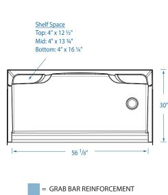
$FEATURES \qquad \hbox{Dimensional Tolerance} \pm \text{\%".} \ Dimensions needed for site preparation should be measured from the unit. Stream 33 assumes no responsibility for preparatory work.}$
