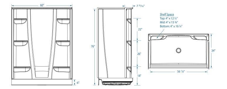
FEATURES Dimensional Tolerance ± %". Dimensions needed for site preparation should be measured from the unit. Stream33 assumes no responsibility for preparatory work.
