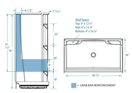
$FEATURES \qquad \hbox{Dimensional Tolerance} \pm \ensuremath{\$''}. \hbox{Dimensions needed for site preparation should be measured from the unit. Stream33 assumes no responsibility for preparatory work.}$
