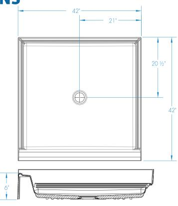
FEATURES Dimensional Tolerance ± %". Dimensions needed for site preparation should be measured from the unit. Stream33 assumes no responsibility for preparatory work.
