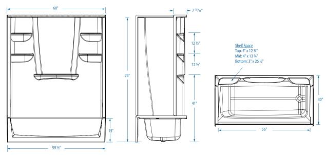
FEATURES Dimensional Tolerance ± %". Dimensions needed for site preparation should be measured from the unit. Stream33 assumes no responsibility for preparatory work.
