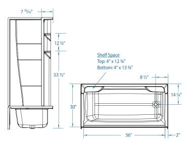
FEATURES Dimensional Tolerance ± 36". Dimensions needed for site preparation should be measured from the unit. Stream33 assumes no responsibility for preparatory work.
