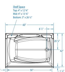
FEATURES Dimensional Tolerance ± 3/". Dimensions needed for site preparation should be measured from the unit. Stream33 assumes no responsibility for preparatory work.
