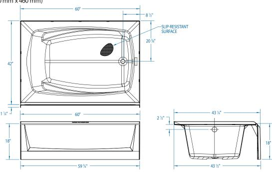
FEATURES Dimensional Tolerance ± 1%. Dimensions needed for site preparation should be measured from the unit. Stream33 assumes no responsibility for preparatory work.
