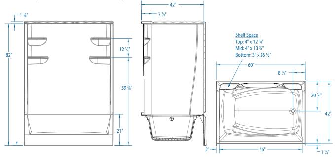
FEATURES Dimensional Tolerance ± 3/6". Dimensions needed for site preparation should be measured from the unit. Stream33 assumes no responsibility for preparatory work.
