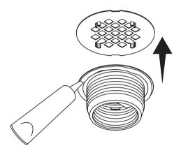
6 Verify that the drain pipe is centered inside the rubber gasket.
