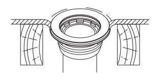
**3** Insert the drain body into the fixture.
