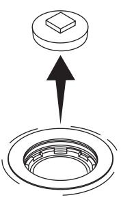
Press the strainer firmly into the drain body.
