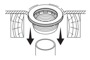
2 Remove the strainer. Apply plumber's putty under the flange.
