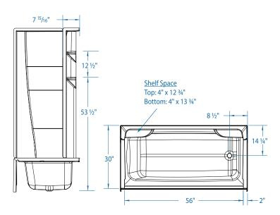
$FEATURES \qquad \text{Dimensional Tolerance} \pm \%. \text{Dimensions needed for site preparation should be measured from the unit. Stream33 assumes no responsibility for preparatory work.}$
