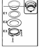
E. Take the remaining portion of the mount assembly, that was put aside. From under the sink insert the Fiber Gasket (E1), then the Support Flange (E2), and then the Upper Mount Ring (E3).
