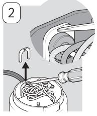
2. Using a flathead screwdriver or needle nose pliers, remove clip from strain relief portion of the cord.
