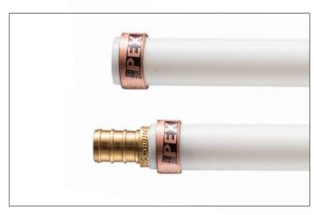
2. Install PEX-B Crimp Ring onto OD of tubing. Install PEX-B fitting fully into tube end.
