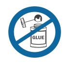
Glue/Primers/Chemicals: PPSU fittings should be protected from harmful chemical exposure. Do not allow any oils to contact PPSU fittings.
