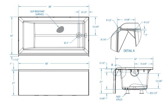
FEATURES Dimensional Tolerance ± 3/8". Dimensions needed for site preparation should be measured from the unit. Stream33 assumes no responsibility for preparatory work.
