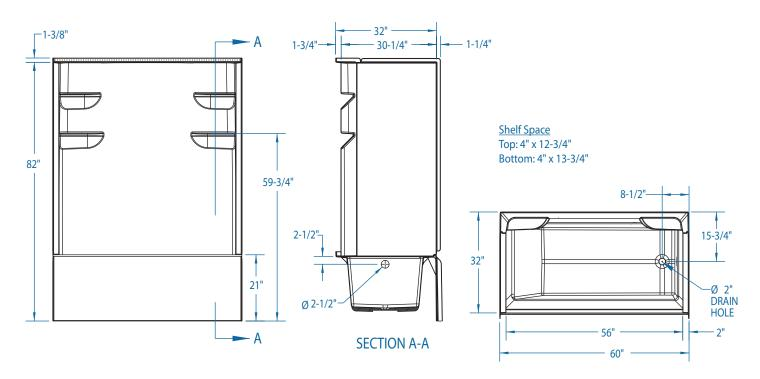
FEATURES Dimensional Tolerance ± 3/8". Dimensions needed for site preparation should be measured from the unit. Stream33 assumes no responsibility for preparatory work.
