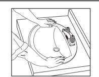
After checking fit and alignment, turn lavatory upside down and apply a generous portion of sealant around the underside of the rim near the edge. Carefully lower lavatory in place, align with marks made earlier, and press down firmly. Allow sealant to set before connecting supplies and drain.
