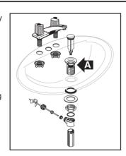
Before applying the sealant, place the lavatory temporarily into the cutout. Check for alignment and clearance. Then mark the lavatory and countertop in several places as a guide for the installation location.
